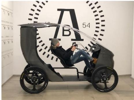
The vehicle is registered as a cargo ebike to be used in bike lanes and car free areas. It's required to peddle and has an ebike 250-500 W engine with max speed of 25km/h. The window and roof give substantial weather protection, and side doors can be added.
